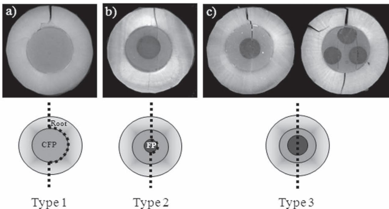
Fig. 6 Typical failure images of RCFP after diametral compression test: a) Failure occurred at interface between root and CFP (Type 1); b) Failure occurred at interface between core composite resin-FP (Type 2); and c) Failure occurred through FP (Type 3). Dotted line indicates propagation line of crack along which fracture occurred.
