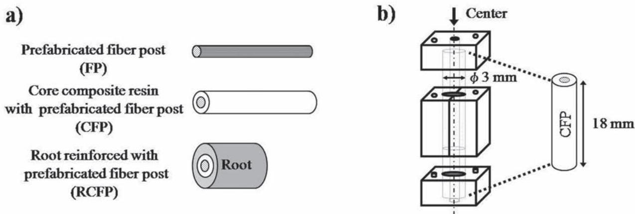
Fig. 1 (a) Three types of specimens, either prefabricated (FP) or fabricated (CFP and RCFP). (b) Metal mold to prepare the specimens (CFP).
