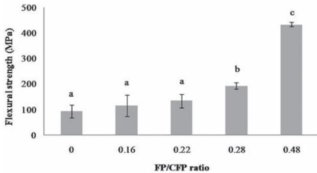
Fig. 2 Flexural strengths of CFPs with different FP/CFP ratios. Different letters indicate statistically significant differences ( $p < 0.05$ ).
