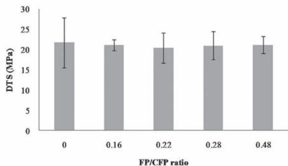
Fig. 5 DTS results of RCFPs with different FP/CFP ratios. No significant differences were observed between any groups ( $p>0.05$ ).
