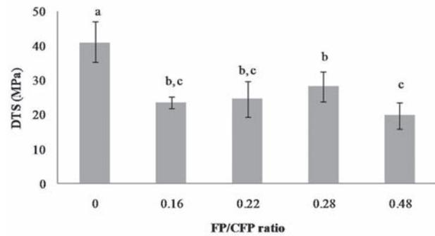
Fig. 3 DTS results of CFPs with different FP/CFP ratios. Different letters indicate statistically significant differences ( $p < 0.05$ ).
