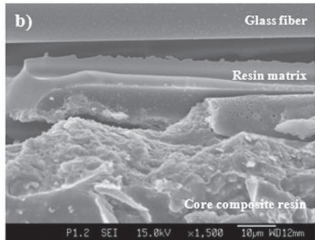
Fig. 4 Typical fracture image of FP after diametral compression test: (a) Optical microscopy revealed fracture through FP which broke the specimen into two. Failure through FP was predominant in all groups; and (b) Fracture between glass fibers and resin matrix in FP.
