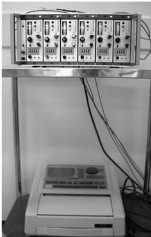
Fig. 1 High-response dynamic strainmeter DPM-612B; oscillographic recorder RDM-100A
