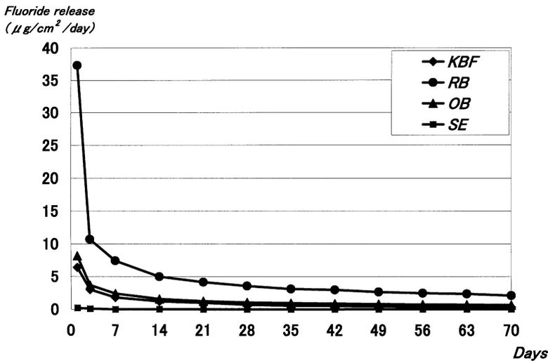
Fig. 2 Changes in fluoride release from each material as a function of time.
