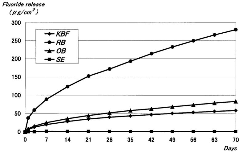
Fig. 1 Cumulative amounts of fluoride release from each material over 70 days.
