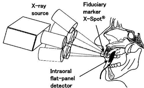
Fig. 1 Schematic presentation of component projections for obtaining TACT base images. A fiducial marker is attached at the buccal surface of the oral mucosa. Four to six exposures are made from different directions while the small flat-panel detector is held in the oral cavity.
