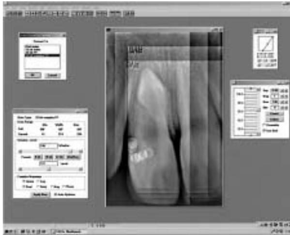
Fig. 2 A selected screen of the TACT Workbench. The tool box, “Clinical TACT slice control”, enables the operator to control the position and the interval of the reconstructed sectional images.
