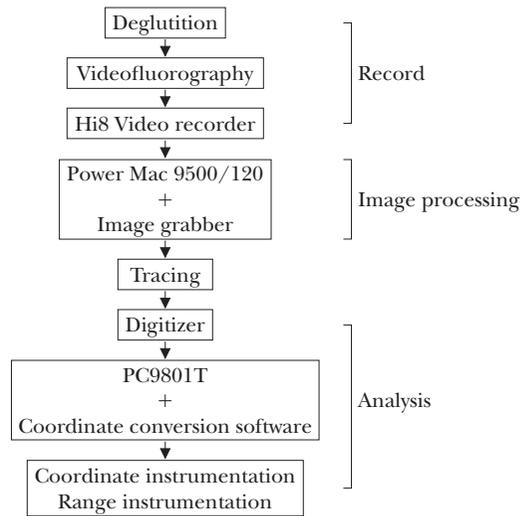
Fig. 2 Block diagram of the analysis method
