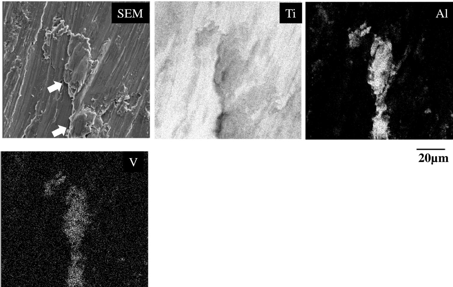
Fig. 6 X-ray image analysis of lower Ti-4 specimen when Ti-alloy (Ti-6Al-4V) was used as an upper specimen.
