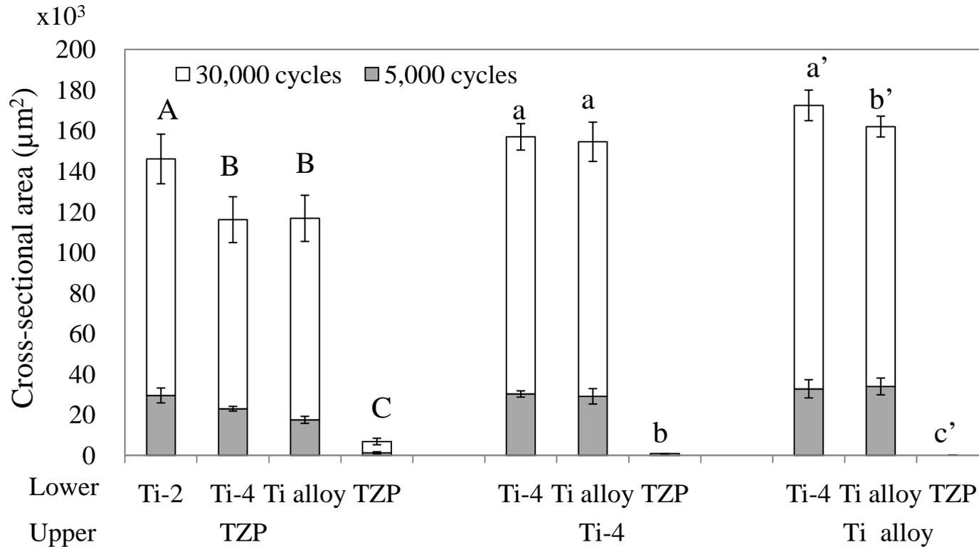
Fig.4 Cross-sectional area of lower specimens against various upper specimens under 2-body wear test. Identical letters indicate no significant difference ( $p > 0.05$ ).
