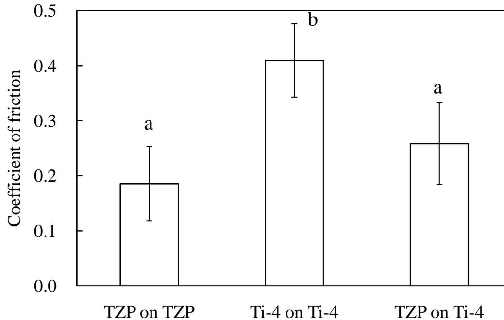
Fig. 2 Coefficient of friction between TZP/TZP, Ti-4/Ti-4 and TZP/Ti-4. Identical letters indicate no significant difference ( $p>0.05$ ).
