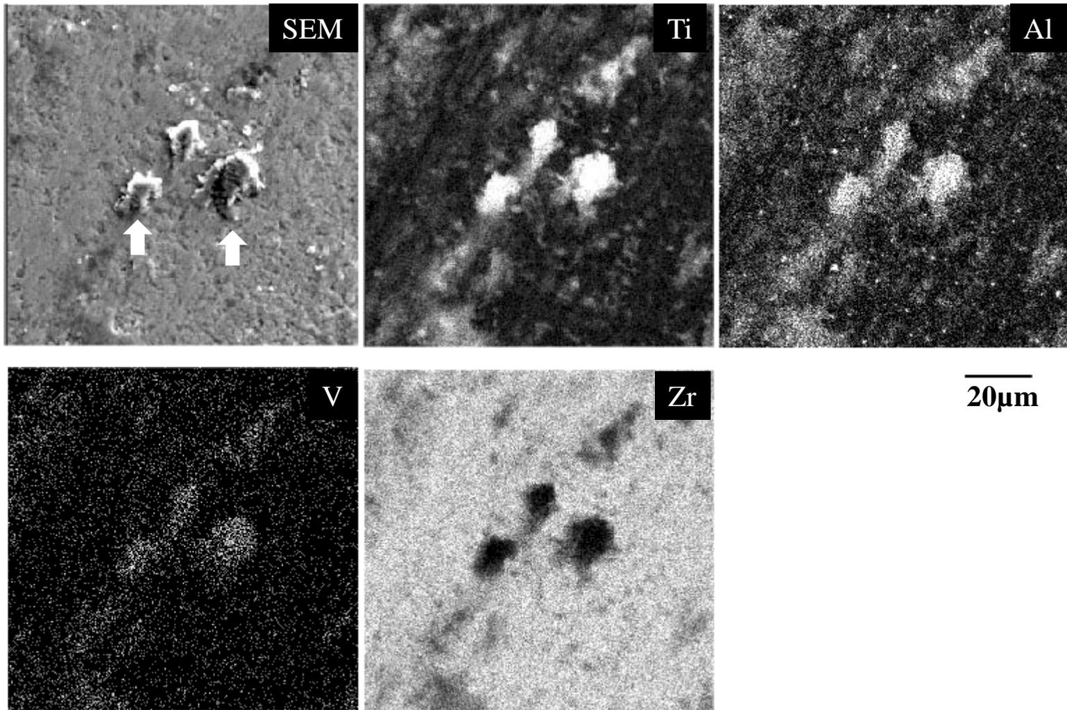
Fig. 5 X-ray image analysis of lower TZP specimen when Ti-alloy (Ti-6Al-4V) was used as an upper specimen.
