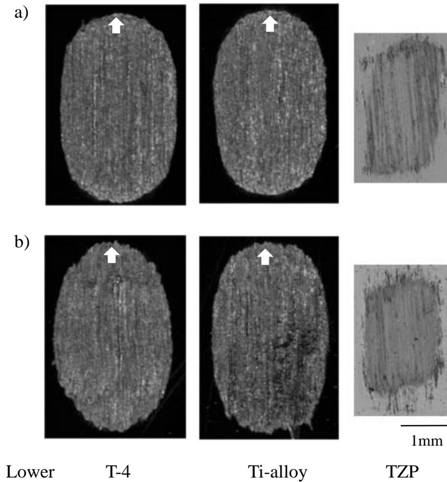
Fig.3 Typical OM images of worn surfaces of lower specimens at 30,000 cycles against upper specimens of a) TZP and b) Ti-4.
