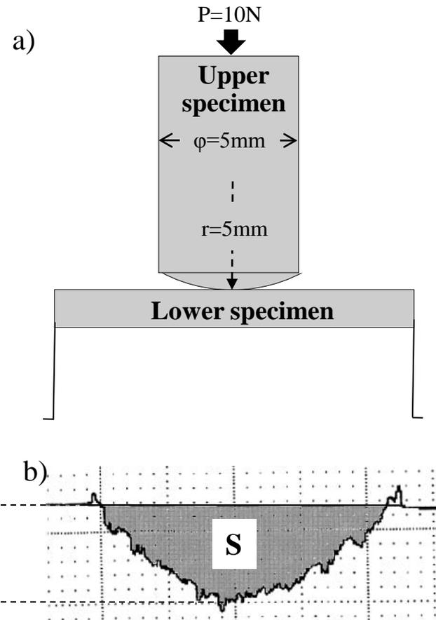
Fig 1 Schematic illustrations of the wear test (a), and the cross section of the worn specimen (b), S: cross-sectional area
